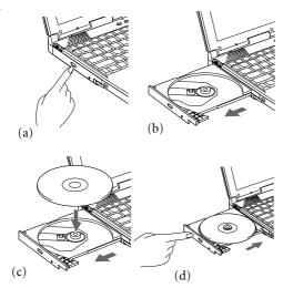
Figure 4-7 Loading/Ejecting Media
